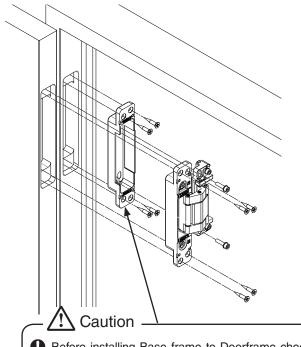
Before installing Base frame to Doorframe check the mounting direction by coupling it with Hinge main body.
