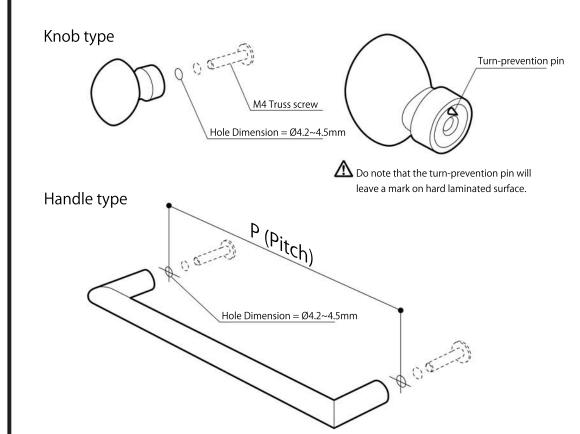
A Please ensure that pitch dimension is correct. Otherwise, the hole that was opened wrongly will be seen, or pull knob cannot be installed properly, etc.
