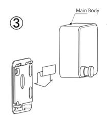
1. Slide Main Body onto Connector from the top.
