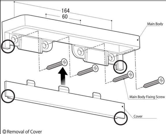
Insert minus screwdriver head into groove and push Cover out.
