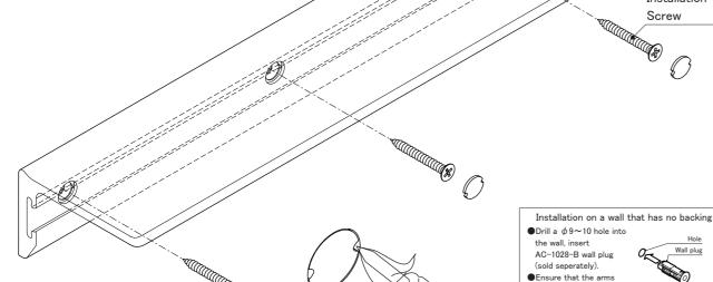
©Removing Screw Cap Insert a pointed object into the hole and pry it out. ※Do it with both holes if needed.
